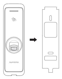
**3** Assemble BioEntry W2 with the bracket by rotating the product fixing screw.
